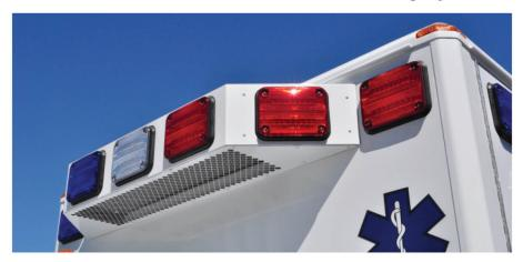
The Wheeled Coach Cool-Bar<sup>™</sup> is the latest innovation from Wheeled Coach, designed to allow the use of an auxiliary A/C condenser without compromising the safety of the front mounted warning lights. Cool-Bar uses a high volume condenser for more efficient patient air conditioning while enhancing safety with two angled warning lights.
