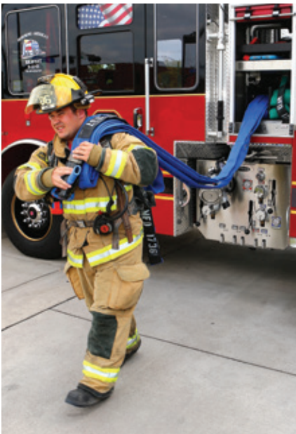
Lower crosslay height for easier hose removal
