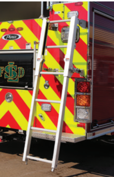
Angled folding ladder for a safer climb
