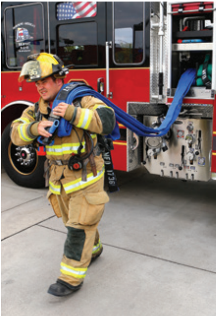
Lower crosslay height for easier hose removal
