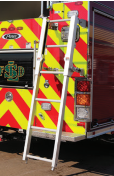
Angled folding ladder for a safer climb
