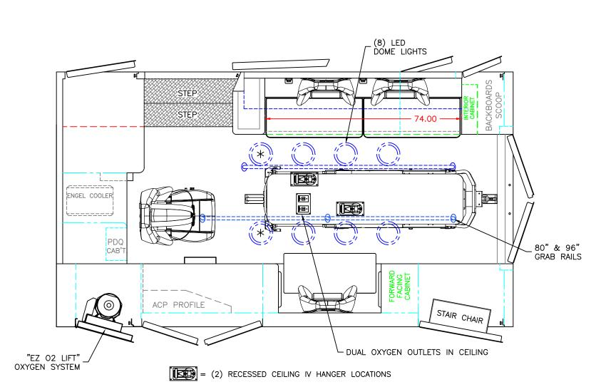
\* = (2) ANTENNA BASES LOCATED OUTBOARD OF DOME LIGHTS WITH COAX SERVICE LOOP
