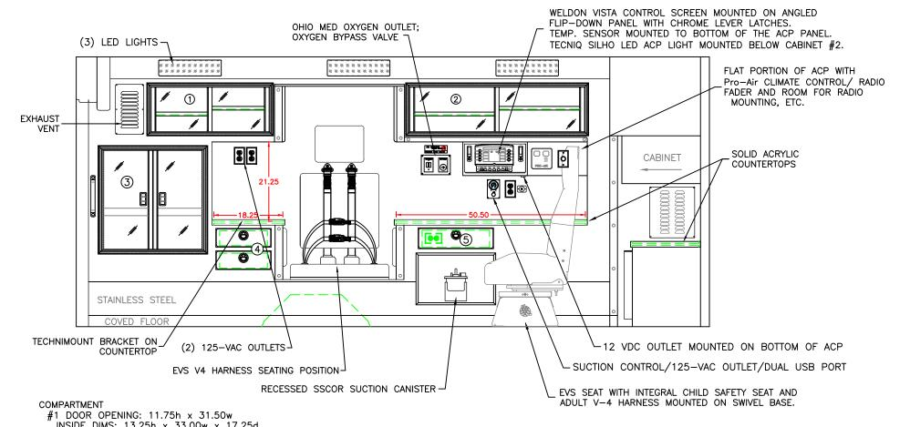
INSIDE DIMS: 13.25h x 33.00w x 17.25d (1) ADJ SHELF EACH SIDE OF CENTER DIVIDER SLÍDING POLYCARBONATE DOORS TOTAL CABINET WEIGHT RATING = 25 lbs.
