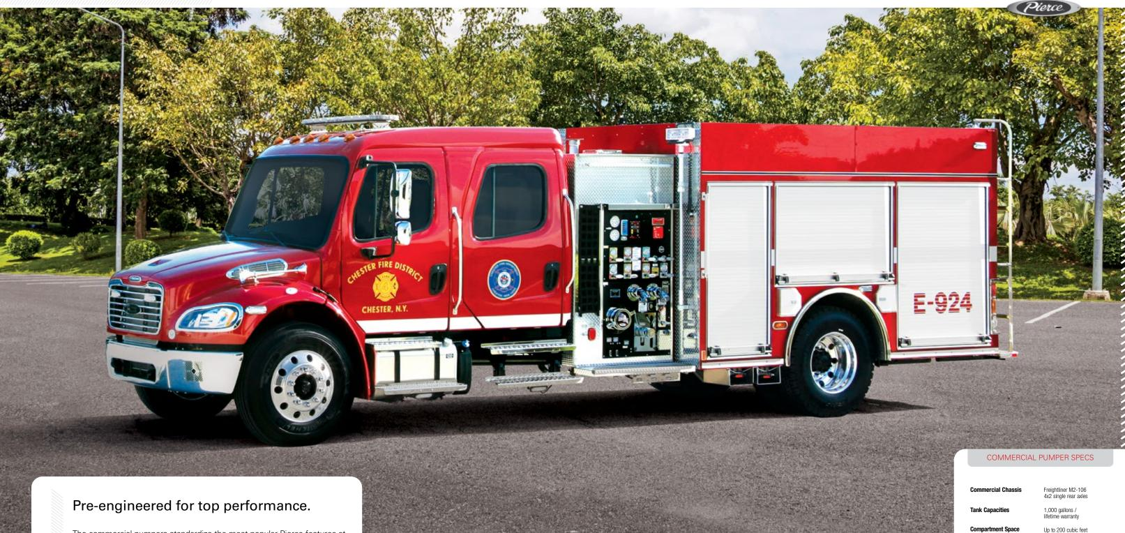
The commercial pumpers standardize the most popular Pierce features at a very competitive price. Standards include an aluminum body with high side spatter painted compartments on each side, LED lights, rollup doors, enclosed ladder storage, wrap-around tail lights, and a full width hose bed.
