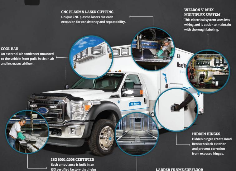
The ladder frame subfloor structure uses extruded tubes on each aisle side for extra support.
