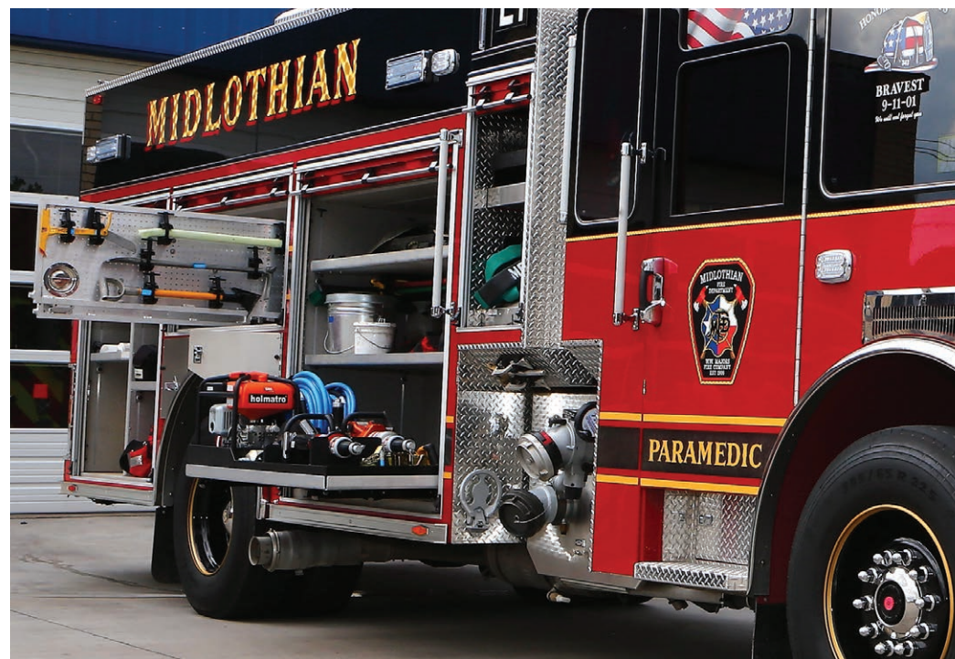
Pierce "jump-off" compartment - provides additional storage due to the unique pump location (traditional pump panels normally occupy this area)
